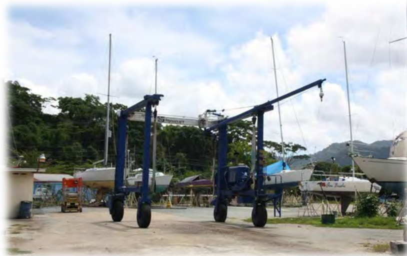
TTS MARINELIFT CAN TAKE VESSELS TO ABOUT 10 TONS
