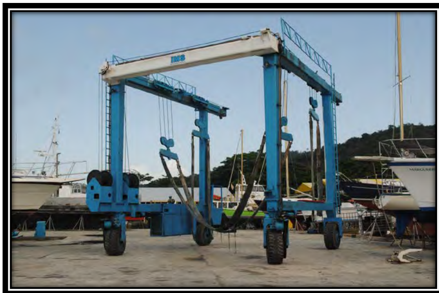
70 TON TRAVELIFT CAN HANDLE MOST BOATS AT IMS
